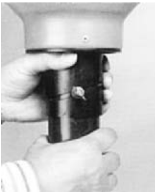
The outlet pipe can be adjusted and the feed regulated directly.
